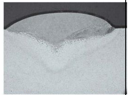
Figure 4 Metallographic cross-section of 0.015-in. filler wire weld shown in Figure 1.
