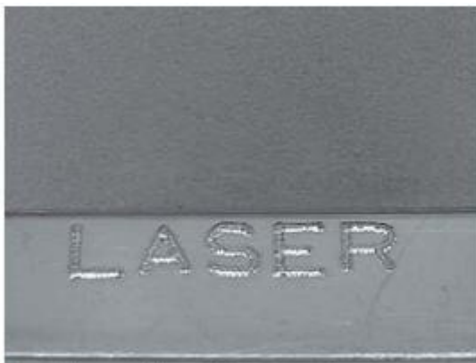
Figure 5 Laser weld repair of an engraving.
