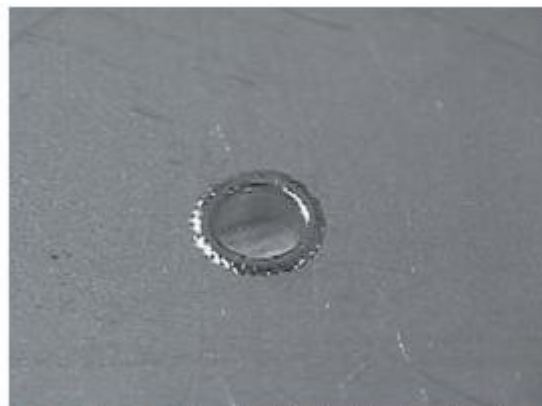
Figure 6 Laser weld repair of the inside diameter of an 1/8-in. hole.
