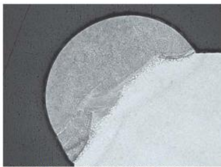
Figure 2 Metallographic cross-section of corner weld shown in Figure 1.
