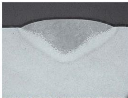
Figure 3 Metallographic cross-section of 0.010-in. filler wire weld shown in Figure 1.
