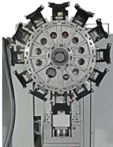
Fast tool change through automatic tool changer with turret type direct pick up
